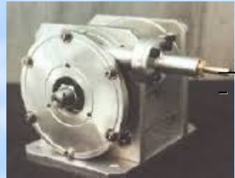
EGG Tesla Turbine 340 kWp Runs on waste heat 177°C to 232°C from exhaust - 650 psig
